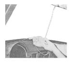
Lubricate the ½" glass grove to allow the glass to find center while installing. Place new rubber on glass making sure that it is placed correctly and fits well. Any problems with fit will show up at this point. Rubber should fit glass without being too loose or too tight. Improper size will pucker or fold in corners. Place chrome strips clip in slots of rubber first. Place 3/16" cord in pinchweld slot of rubber around perimeter to help pull flap over pinchweld.
