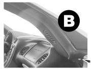
Starting at the bottom of the A-Pillar, carefully pull or pry the push-in pin retainers (FIG. B) from the molded end pieces. Gradually extract the original weatherstrip from the A-pillar channel, ensuring a slow and complete removal.
